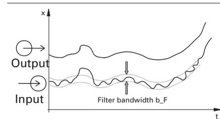
The bandwidth is the adjustable tolerance around the process value in which the filter is active. Measured value changes exceeding the adjusted bandwidth are passed through directly.
