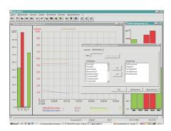
Besides the x/t display, it is also possible to select an x/y display. In this case, up to 6 signals are displayed online over a freely selectable measuring channel.
