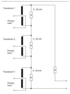
The resistors must be matched in such way that the resulting output signal can be read by the analogue input board from the PLC.
